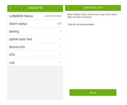
Uplink data test: When LoRaWAN Status on the main page shows connected, but no Data has been transmitted, a real-time message (the default is the current date and time) can be sent to the server through the Uplink Data Test interface of the APP. If the server fails to receive the message, it indicates that the network connection is abnormal.
