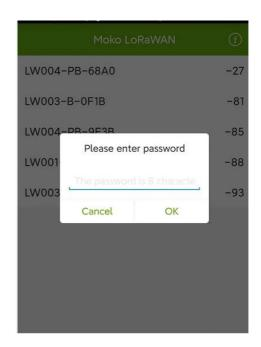
click the device name to connect the device that you want to configure. Then you should enter the password, the default password is "Moko4321".
