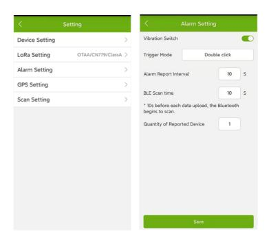
Come into setting interface. In the Alarm Setting page we can get and configure some alarm parameter.
